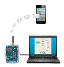
Program either by connecting the units to a PC and using the PC application supplied, or by sending SMS commands from your cellphone
