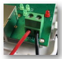
Connect the provided serial cable from the serial connector on the X-series panel to the serial connector on the HYYP IP Connect Module.
