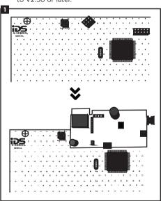
Plug the unit into the expansion connectors on the IDS alarm panel as shown.
