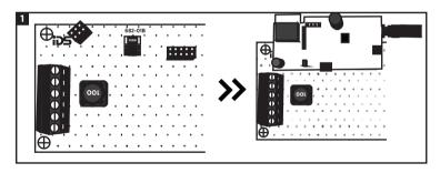
1. Plug the unit into the expansion connectors on the IDS Panel as shown.
